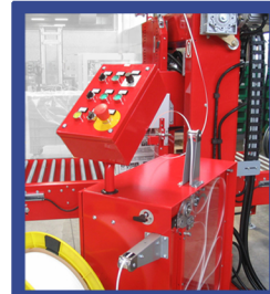
PANNELLO COMANDI OPERATOR PANEL
