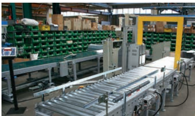
Packaging line with 0875 TR200 and conveyors
